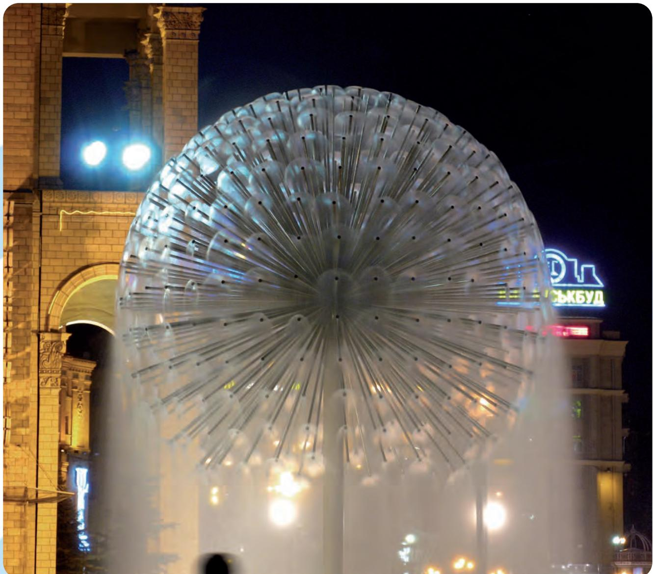
This type of fountain nozzle requires a separate mention, given its special appearance and performance. It could be catalogued as crystalline because each individual jet pipe generates a disc of transparent water, but **the end result is the combination of hundreds of discs that create a remarkable spherical (or semi-spherical) volume**. Furthermore, because it moves a large volume of water, it forms an extremely large column when it falls.
