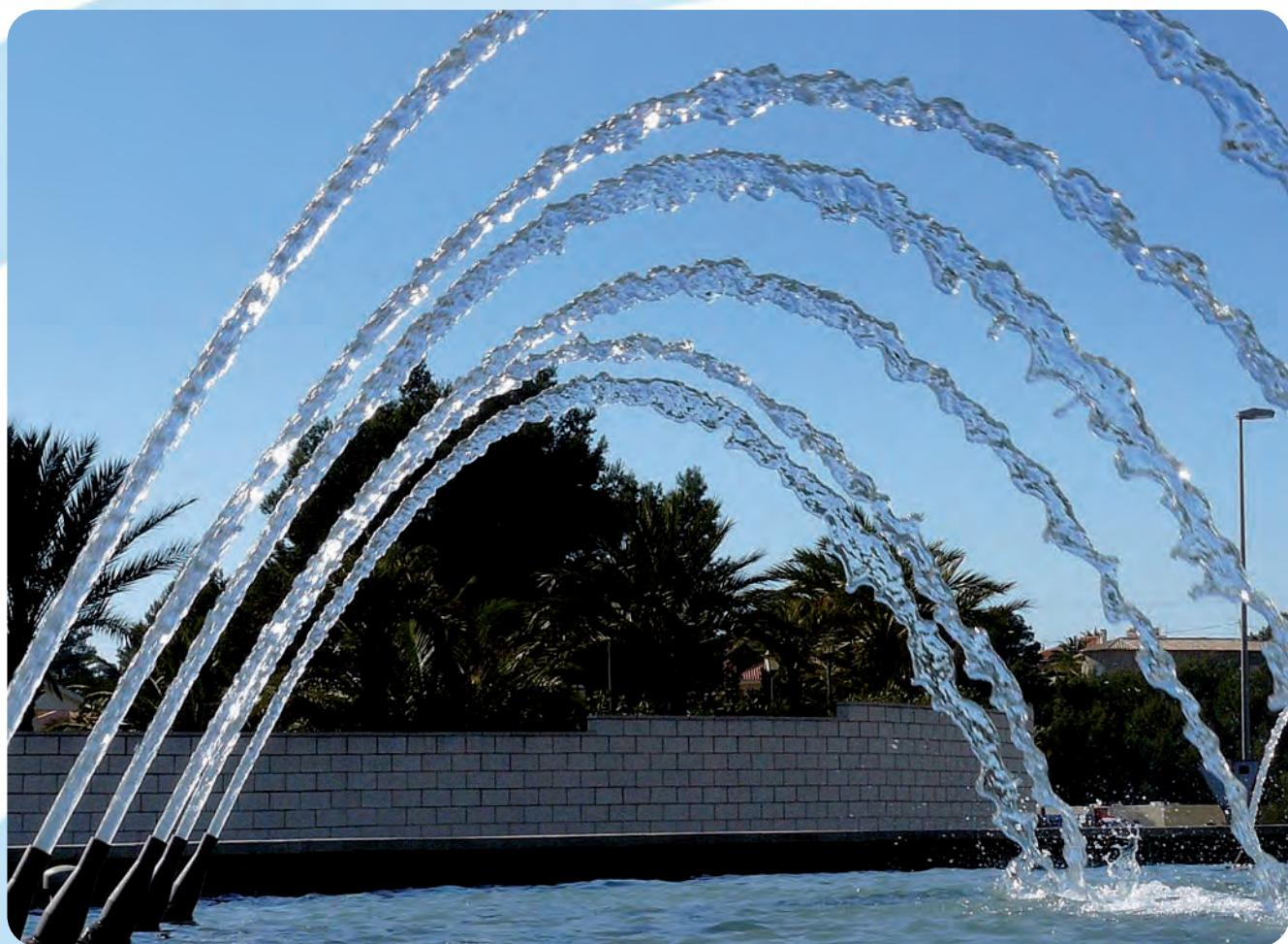
**T**hese fountain nozzles produce a crystalline feature effect in the fountain jets and ensure that its flow inside the jet pipe is laminar. In order to prevent turbulence, all nozzles in the series are fitted with jet disturbers to "calm" the water flow. The aim is to ensure that the water jet is transparent, which means there must be no air inside it. The most representative jet produced by this jet pipe is the crystal-clear jet.
