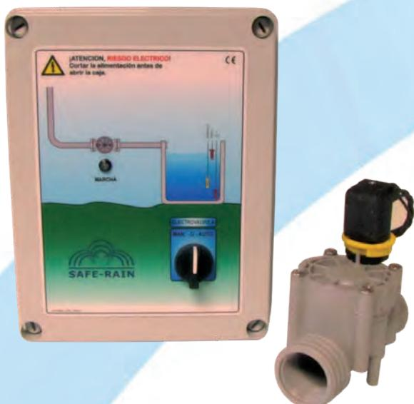
**S**ystem that automatically controls the minimum and maximum water levels of architectural fountains with two electrodes, one for the minimum level and the other for the maximum level. When the minimum water level is reached, the solenoid valve connected to the sensor is opened. It closes automatically when the maximum level is reached.
