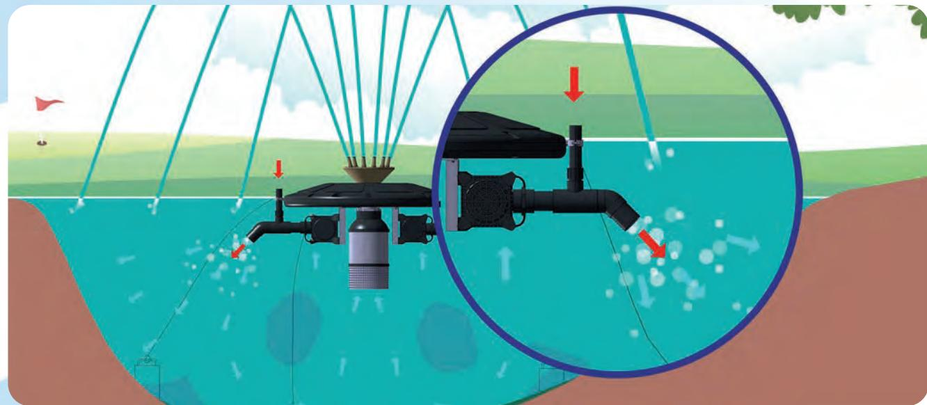
**T**hanks to **water pond aeration system** manufactured by Safe-Rain you could oxygenate the water of any lake, facilitating biological cycles and ensuring the effectiveness of bacterial products that reduce nutrients and clarify water.
