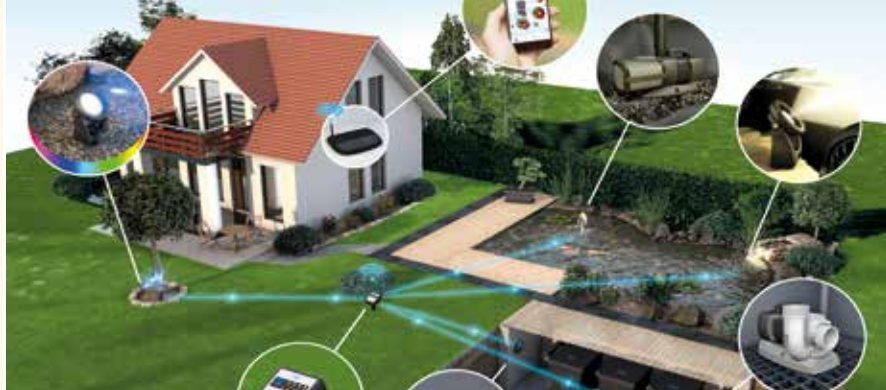
Schematic diagram: InScenio EGC Controller networked with router and EGC-capable OASE devices
