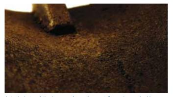
Actual photo of the inner surface of a cast Cascade nozzle. You can notice the bumpy surface that is held responsible for the water height loss and the overall inefficiency of cast nozzles.
