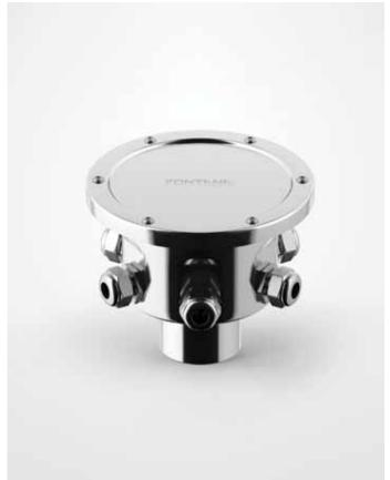
Cable inlets with integral junction box are a unique solution for both watertight, safe & inconspicuous cable transitions into the fountain basin and underwater wire connections, all in one unit. The housing is made of superior quality, corrosion-resistant stainless steel AISI 304 (or 316 on request) and offers sufficient space for effortless electrical connections and passage of cables. All models have a removable cap for easier access.
