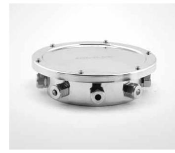
Junction boxes are used for watertight cable connections and disconnections. You can connect submersible pumps, lights, sensors and other electrical devices safely and effortlessly. There is a wide variety of junction boxes to choose from with models with 4 up to 24 waterproof cable glands for all types of cables. The high quality and corrosion resistant housing is made of AISI 304 stainless steel (or 316 on request) and the removable cover provides extra usability.
