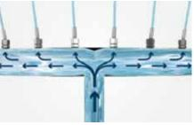
Flow Diverters on every inlet and Flow Straighteners on every nozzle to achieve optimum performance and water efficiency
