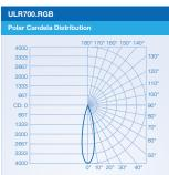
Photometric Test on White (R,G,B at 100%) Beam Center: 3978 cd Multipliers: Red 0.25, Green 0.65, Blue 0.1
