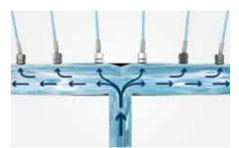
Flow Diverters on every inlet and Flow Straighteners on every nozzle to achieve optimum performance and water efficiency
