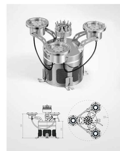
This fountain kit comes with two types of pumps: 300W & 700W offering max flow of 2.36 l/s and 3.89 l/s respectively. It is ideal for medium scale applications with a wide variety of nozzles for every type of water effect. You can also choose another nozzle to combine it with this fountain kit.
