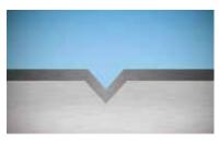
FIG. 3 The protective coating is quickly restored through the rapid self-repairing quality of the chromium rich film.
